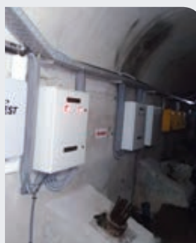
Manual reading boxes and data acquisition unit
