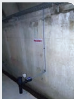
Piezometers equipped with a pressure sensor
