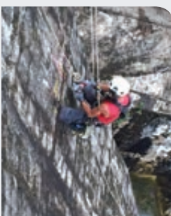
Testing on the downstream surface of buttresses by professional rope access technicians
